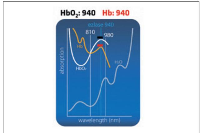
**Fig 11** Schematic presentation showing absorption of 940-nm diode laser compared to other wavelengths.
