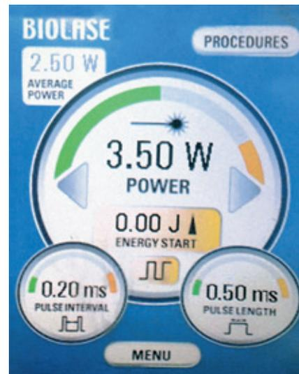
**Fig 3** Laser settings for debridement of granulation tissue and pocket epithelium: 3.5 W pulsed mode with a pulse length 0.50 ms and a pulse interval of 0.20 ms.
