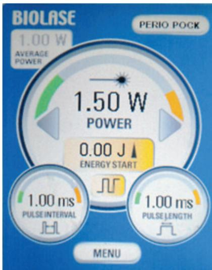
**Fig 2** Laser settings for pocket disinfection: 1.5 W with pulse interval of 1.00 ms and pulse length of 1.00 ms.
