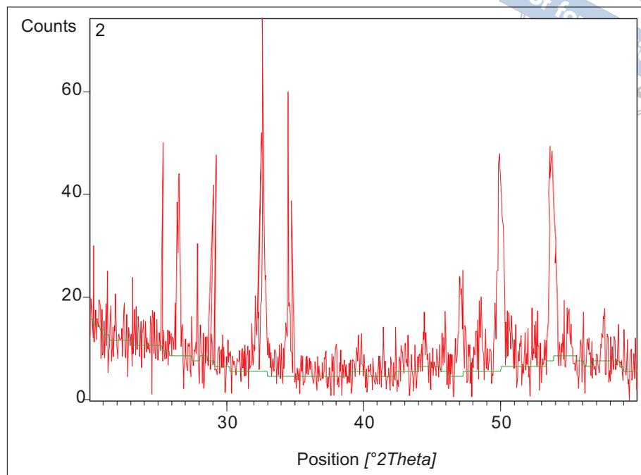
**Fig 4** Irradiation with laser plus fluoride application revealed the presence of fluorapatite, which was not seen in any other groups.
