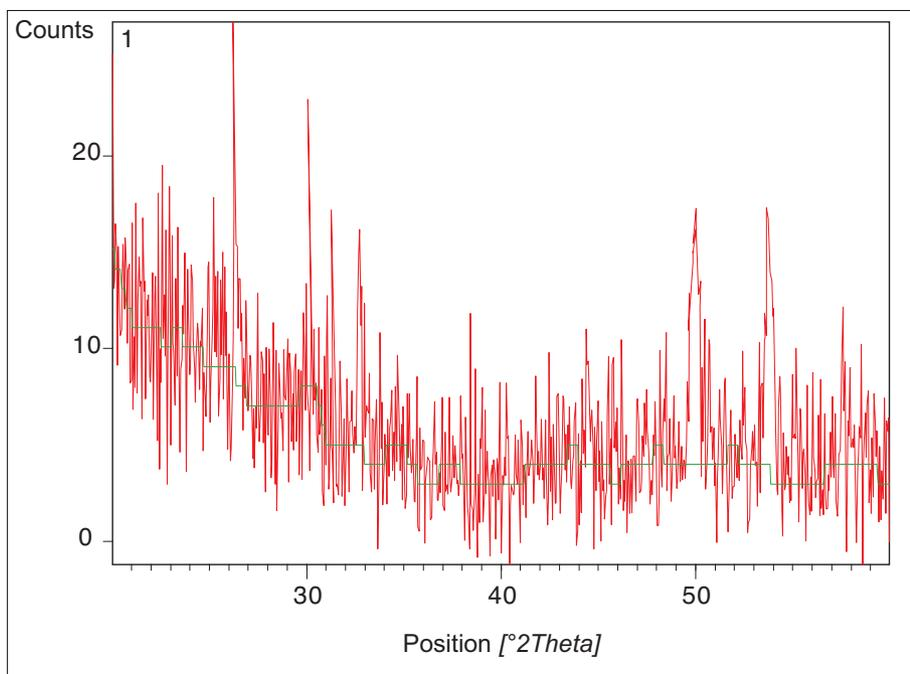
**Fig 2** X-ray diffraction pattern of the group treated with fluoride alone also showed the presence of hydroxyapatite crystals.
