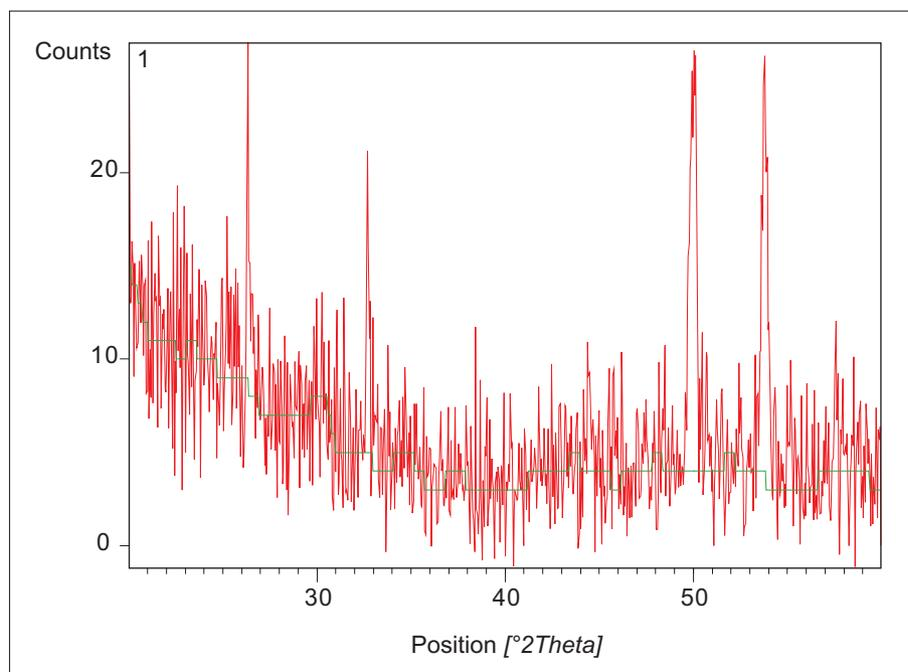
**Fig 1** X-ray diffraction pattern of the control group revealed the presence of hydroxyapatite crystals.
