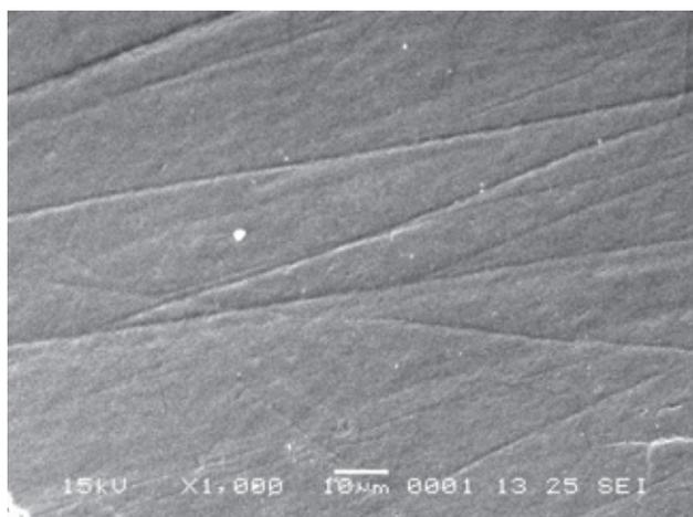
**Fig 5** SEM of control specimen: untreated enamel surface.
