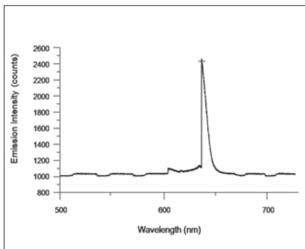
**Fig 3** Emission spectrum of the red LED.
