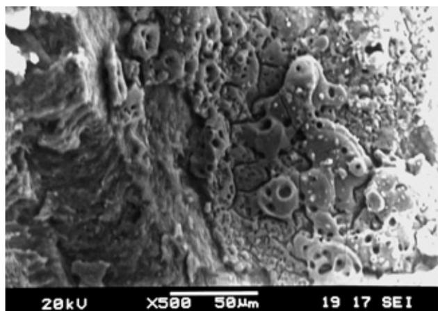
**Fig 9** Sample of group 4 with melting dentin resulted from 1 W and 2 s and black Ink of Nd:YAG laser treatment.
