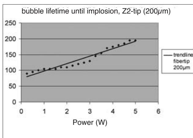
**Fig 13a** Lifetime of the vapor bubble in a free water situation until implosion, fiber Z2, 20 Hz.
