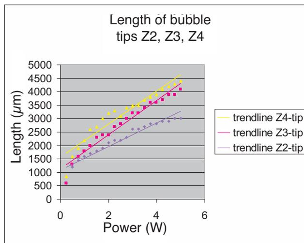
**Fig 8** Length of the bubble vs power on the display of the laser at 20 Hz.
