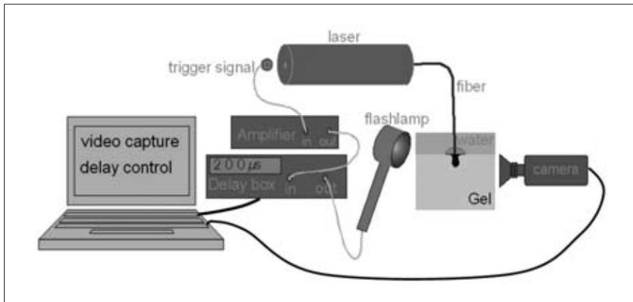
Fig 1 Optical setup.
