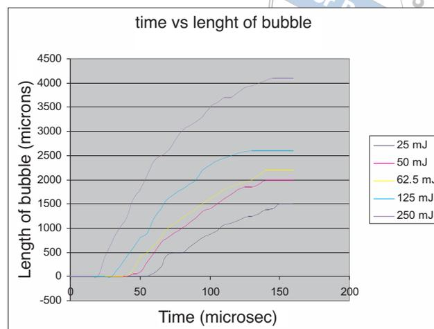
**Fig 9** Development of bubble length in time for a 400- $\mu\text{m}$  fiber for energies from 25 to 250 mJ.
