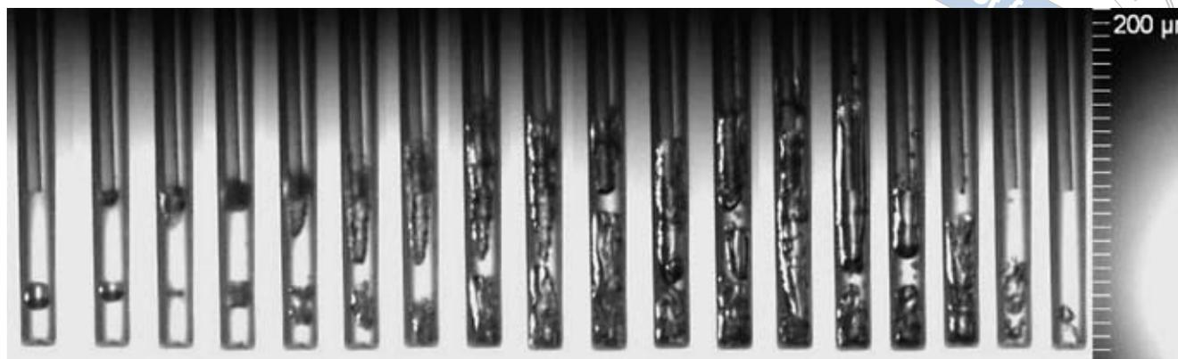
**Fig 12** Captured images of expanding and imploding vapor bubble inside the cylindrical root canal model from 0 to 1200  $\mu$ s after the onset of 50 mJ pulses.
