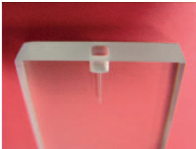
**Fig 2** Glass block with root canal and artificial pulp chamber.
