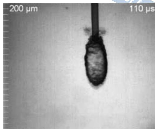
**Fig 5** Example of a captured image of an expanding bubble.
