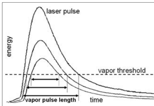
**Fig 14** The temporal pulse profile of an Er,Cr:YSGG laser at different energy levels. Note that at higher pulse energies the vapor pulse length is increased, since the vapor threshold remains constant.
