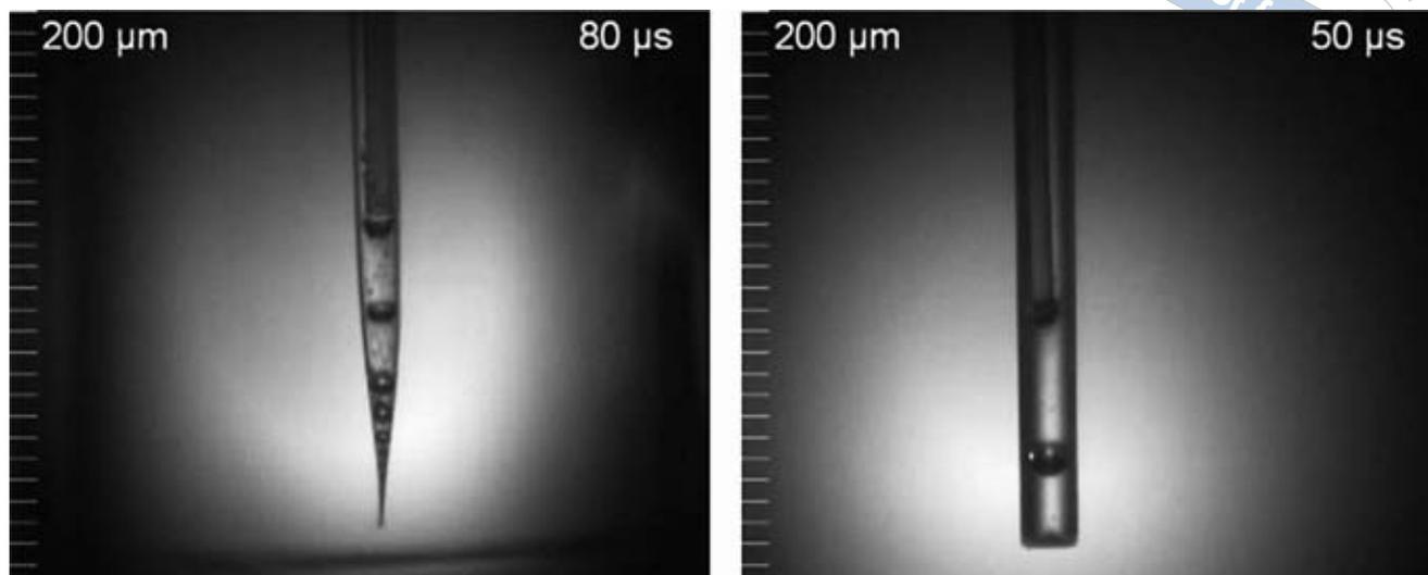
**Fig 10** Examples of captured images of a bubble at the start of expansion in the conical (left) and cylindrical (right) root canal model.
