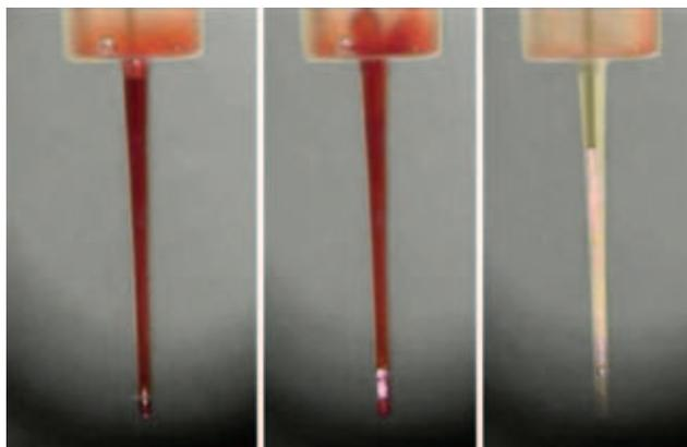
**Fig 4** The left panel shows the root canal model filled with red dye and clear fluid on top in the artificial pulp chamber. At the first few laser pulses (12.5 mJ at 20 Hz), a cloud of red dye ejects into the pulp chamber (middle panel). After 3 s, the red dye in the canal has been replaced by clear fluid (right panel).
