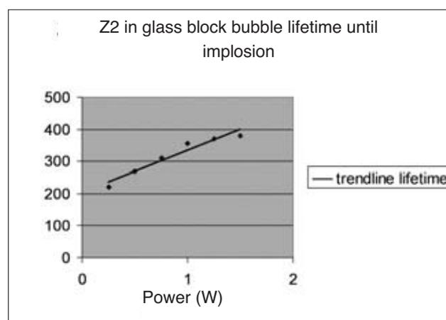
**Fig 13b** Lifetime of the vapor bubble in a glass block until implosion, fiber Z2, 20 Hz.
