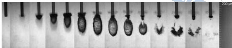
**Fig 7** Captured images of expanding and imploding vapor bubble induced by 125 mJ (top) and 250 mJ (bottom) pulses at 20 Hz. The sequences of frames from left to right show the dynamics in time after start of the pulse at 0, 25, 50, 80, 100, 150, 205, 265, 320, 355, 375 and 400  $\mu$ s.
