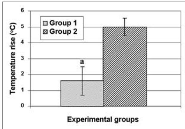
**Fig 1** Graphic representation of the temperature rise (°C) inside the dental pulp chamber during the irradiation with the gated-pulsed (group 1) and continuous-wave modes (group 2). (a) Significantly smaller than group 2 ( $p < 0.05$ ).
