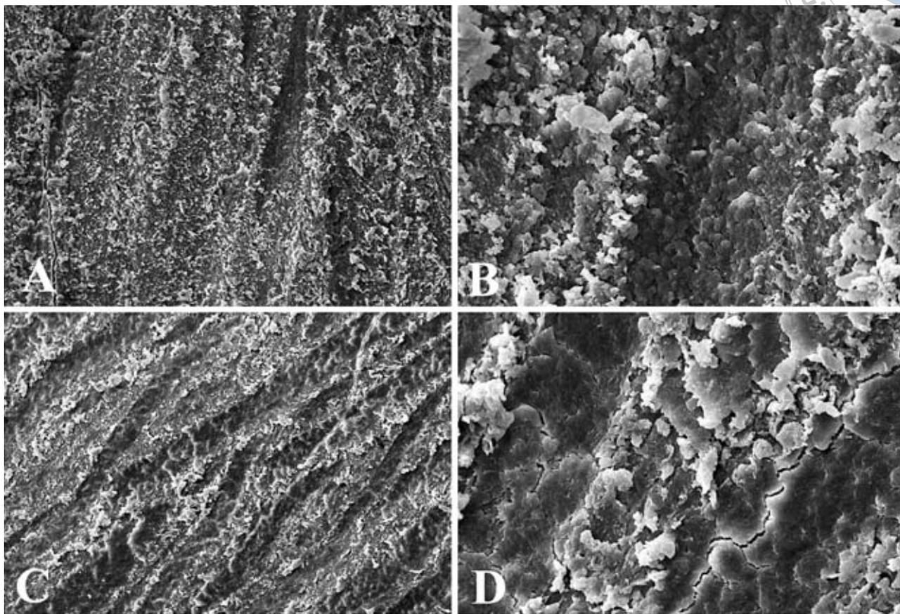
**Fig 2** Scanning electron micrographs of the root fragments treated with the high-power diode laser with the gated-pulsed mode (A, B) and continuous-wave mode (C, D). Original magnification 200X (A, C) and 1000X (B, D).
