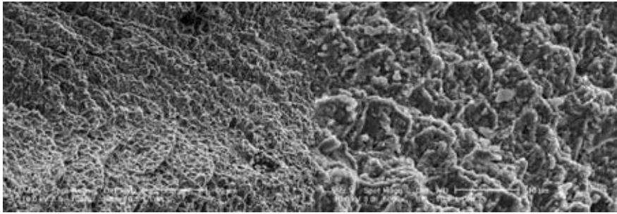
**Fig 3a** (left) Low magnification SEM of laser-ablated enamel demonstrating the absence of a smear layer.
