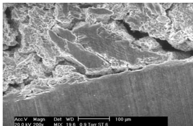
**Fig 14** Sample D4, Er,Cr:YSGG, 1.5 W, detail, 200X.
