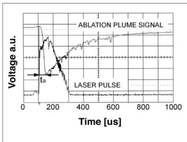
**Fig 1** The evolution of the ablation plume signal during and after the Er: YAG laser pulse.
