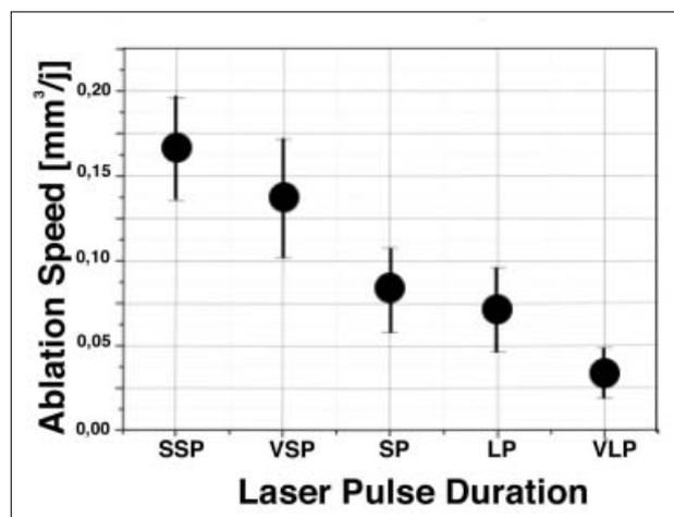
**Fig 2** Dependence of the ablation speed on the Er: YAG (Fidelis) pulse duration mode. Standard erbium lasers achieve ablation speeds of ca 0.057 mm<sup>3</sup>/J. A much higher ablation speed of 0.165 mm<sup>3</sup>/J is achieved by the shortest SSP laser mode.
