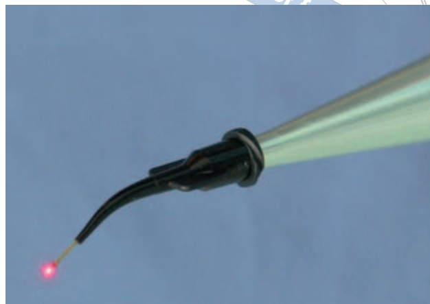
Fig 2 Optical fiber of 300 µm diameter mounted on the hand-piece with plastic tip.
