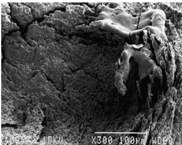
Fig 4e Representative enamel surface of the 300 mJ/pulse samples. Next to the irregular and ablated surface an area of vitrification can be seen.
